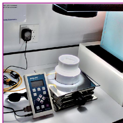
Figure 1. The experimental set-up to qualitatively assess potential protective properties of finished goods products against full solar radiation and its VIS plus IR portion.
