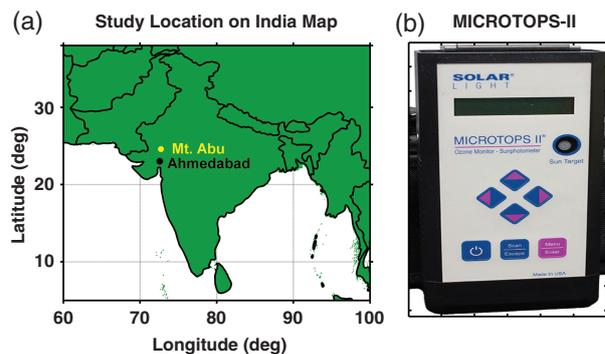
Figure 1. (a) Location of Ahmedabad and Mount Abu in India and (b) a photograph of the MICROTOPS II ozonometer instrument. [Colour figure can be viewed at [wileyonlinelibrary.com](http://wileyonlinelibrary.com)].
