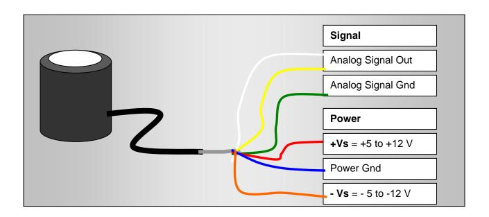
It is essential for proper operation to connect the RED wire to the positive power supply and the ORANGE wire to the NEGATIVE power supply. The BLUE wire is the POWER ground.
