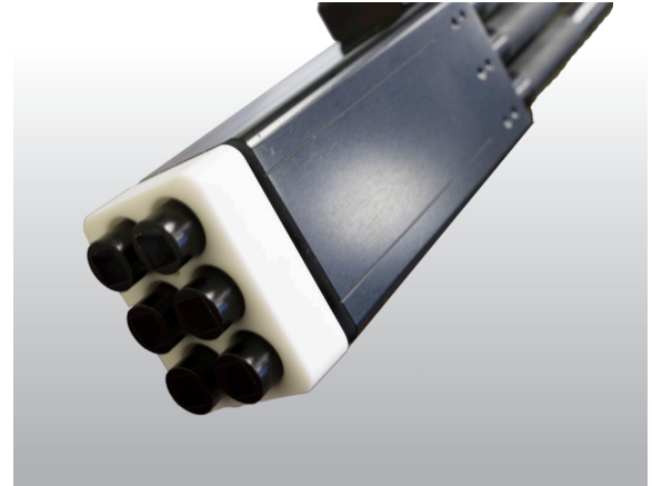
Figure 1. Illustrates advanced optical system for SPF testing with Teflon endpad (White) P/N SL-06163.
