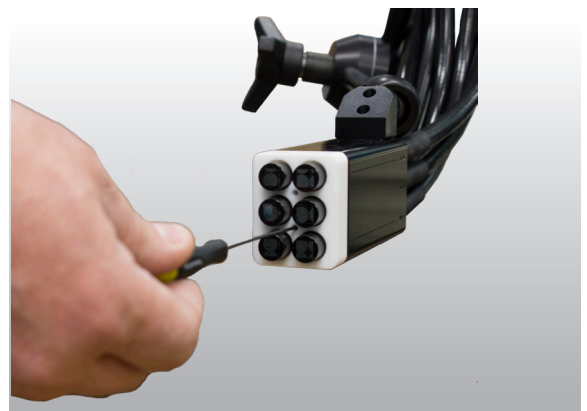
Figure 3. Illustrates the two screws that adjust the standoff distance between the teflon endpad and LLG homogenizer
