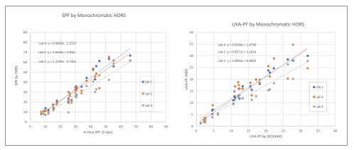
Figure 7. Results from the three monochromatic DRS devices for the 25 test samples for SPF and UVA-PF compared with in vivo SPF and both in vivo and in vitro UVA-PF (ISO 24443) results.
