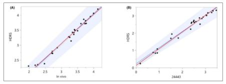
Figure 9. Passing-Bablok plots combining results of all 4 laboratories for SPF (A), and UVA-PF (ISO24443) (B). The blue bands depict the 95% confidence interval for the regression. Note the data are presented in the In transformed domain as the data are log-normally distributed.
