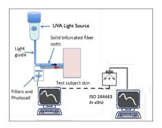
Figure 5. Schematic depiction of polychromatic DRS system for direct measurement of UVA-PF values of sunscreen on human skin. The UVA-PF values are used to scale a full spectrum in vitro absorbance scan of the sunscreen, from which estimates of SPF, and CW can be calculated. Correlations between DRS determined SPFs and UVA-PFs with in vivo results were very strong with slopes close to 1, indicating a 1:1 correspondence between the results. Adapted from Cole et al, (23).
