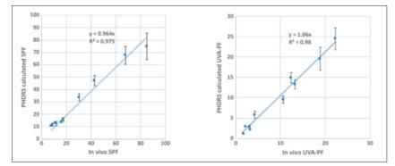
Figure 6. Correlations of SPF and UVA-PFs as determined by PHDRS device and in vivo SPF or UVA-PF (ISO24443) results.
