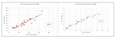
Figure 8. Results from the polychromatic DRS device for the 25 test samples for SPF and UVA-PF compared with in vivo and in vitro UVA-PF (ISO24443) results.
