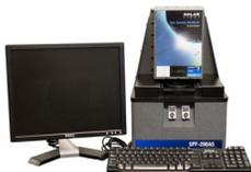
**Ultraviolet Transmittance Analyzers** available as complete integrated turnkey systems to meet the latest ISO24443 requirements.
