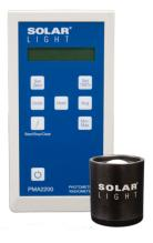
Like the PMA2100, the Model PMA2200 Handheld, Single-Input Radiometer accepts over 85 different PMA-Series sensors measuring UV, Visible and IR wavelengths. Its patented Intelligent Detector Technology combined with Automated Sensor Recognition enables seamless interchange between radiometers and sensors. As with the PMA2100 handheld radiometer, the PMA2200 allows all functions to be operated directly from the keypad with unit of measurement selection, set-points and audible alarms.
