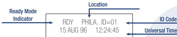
If the name of the selected location is 6 characters long or less it will be displayed in its entirety. Otherwise, only the first 5 characters are displayed followed by two dots indicating continuation. The named locations can be set from a PC via the serial port. If a manually entered (unnamed) location is used then the location name displays “Manual”.
