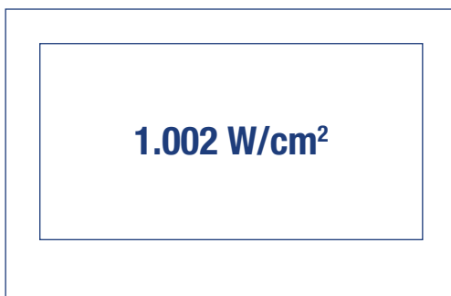
Figure 5 "Data Mode" with Detector Connected - No Integration
